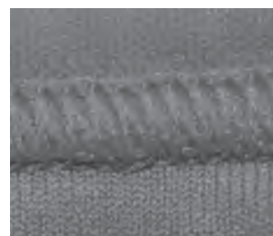
602 Two-needle four-thread coverstitch (back view)
