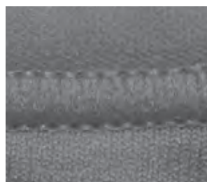
602 Two-needle four-thread coverstitch (face view)
