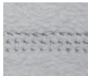
605 Three-needle five-thread coverstitch (back view)
